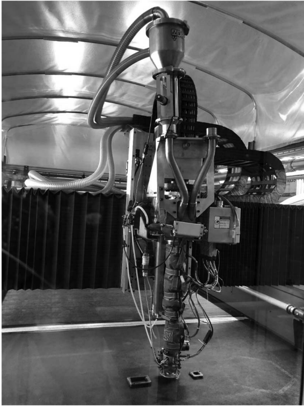
Fig. 2 BAAM extruder during a print
