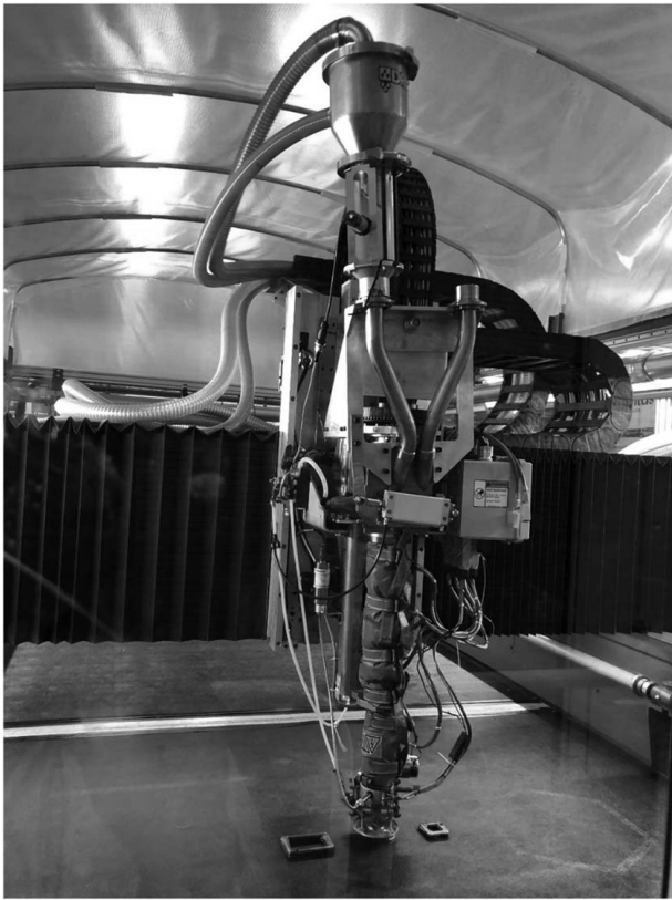
Fig. 2 BAAM extruder during a print
