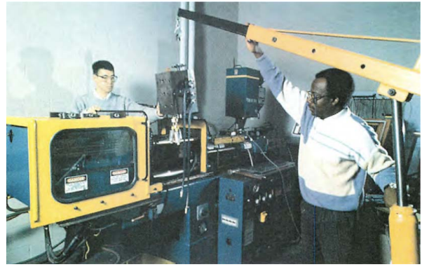
An instrumented mold is installed to study warpage of injection-molded plastics at Cornell CIMP in the 1990s.
