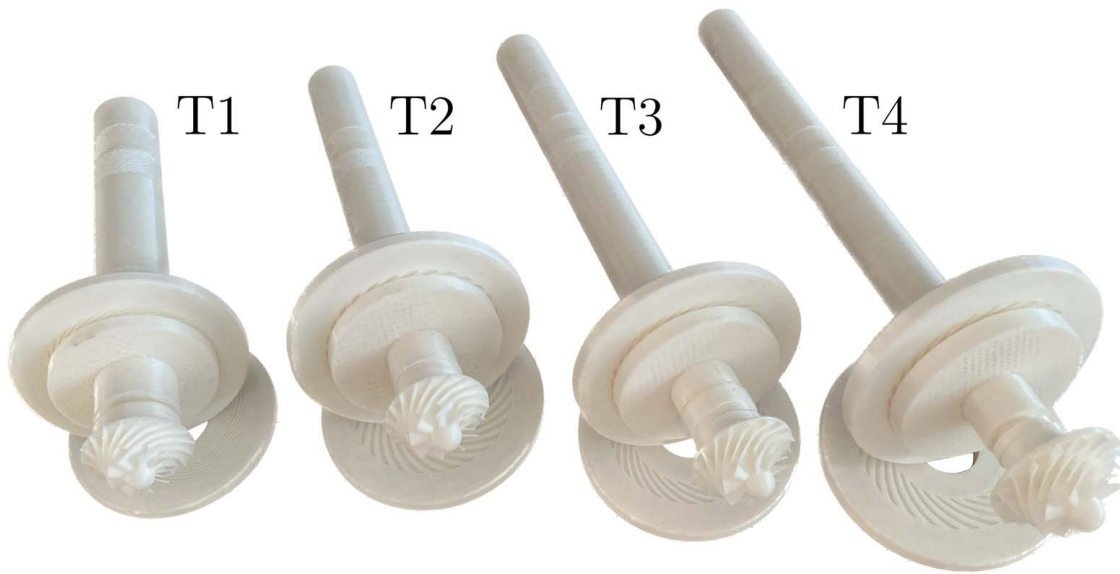
Fig. 6 Three-dimensional printed turbocompressor models T1–T4, each enlarged to 150% scale for enhanced visibility. Key features like groove depths in the herringbone grooved journal bearings (HGJBs) and spiral groove thrust bearings (SGTBs), as well as impeller blade thickness, are amplified to 0.5mm to circumvent the resolution limits of the 3D printing process and to ensure accurate detail reproduction.
