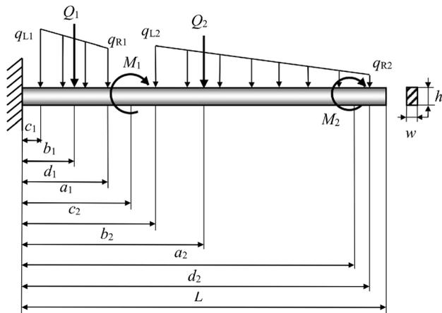
Fig. 3 A cantilever beam system
