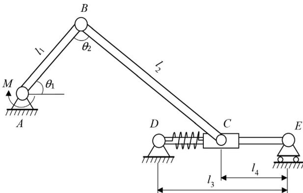
**Fig. 4 A crank-slider system**
