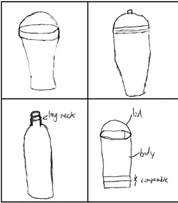
**Fig. 8** A student's initial self-generated concept for the no-spill cup problem (upper left) alongside three concepts they created during brainstorming. The two on the right (both using a domed lid) were coded as similar to the initial concept, and the one below it (with a narrow neck) as dissimilar.
