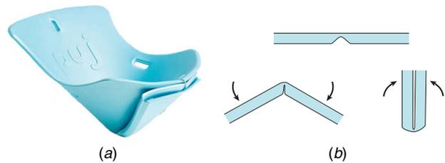
**Fig. 11** The baby bathtub, discussed in Sec. 3.3, uses several stability techniques. (a) The fully folded state is maintained using magnets and adjacent facet interference. (b) Hinge interference prevents the linkage from folding the wrong way (used with permission from PUJ®).
