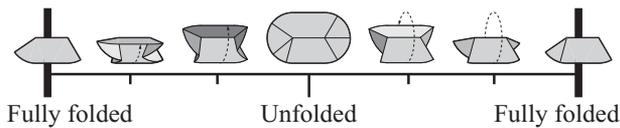
**Fig. 5** A 1D fold-state continuum of a single DOF origami linkage in Fig. 4. Seven fold states along the continuum are shown and marked on the continuum (three are labeled). Dashed arrows are also included on some fold states to help visualize the position.
