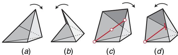
**Fig. 10** Origami linkages (in gray) with (a) and (b) intrinsic and (c) and (d) extrinsic hard stops in (a) and (c) tension and (b) and (d) compression. The added links shown in (c) and (d) represent members that are not part of the original origami linkage.
