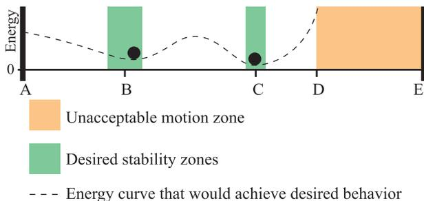
**Fig. 6** An example of how to indicate “desired stability zones” and “unacceptable motion zones,” with an energy curve that achieves the desired behavior. Five example fold states are labeled (A)–(E). Fold states B and C are desired stable fold states. The motion of the origami linkage should not progress past fold state D.
