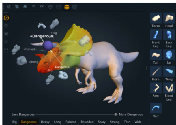
Fig. 1 User interface for assembly based modeling using relative attributes. Used with kind permission of Kalogerakis [18].
