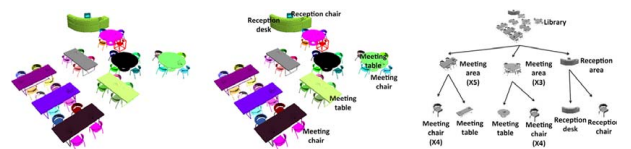
Fig. 2 Input scene mapped with labels and converted into the hierarchical form using probabilistic grammar. Used with kind permission of Liu et al. [20].
