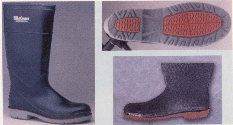
The outer sole of the Flex 3 boot (left) uses a two-step overmolding process to fuse the orange vinyl/elastomer blend (top right) and the harder gray compound (lower right).
