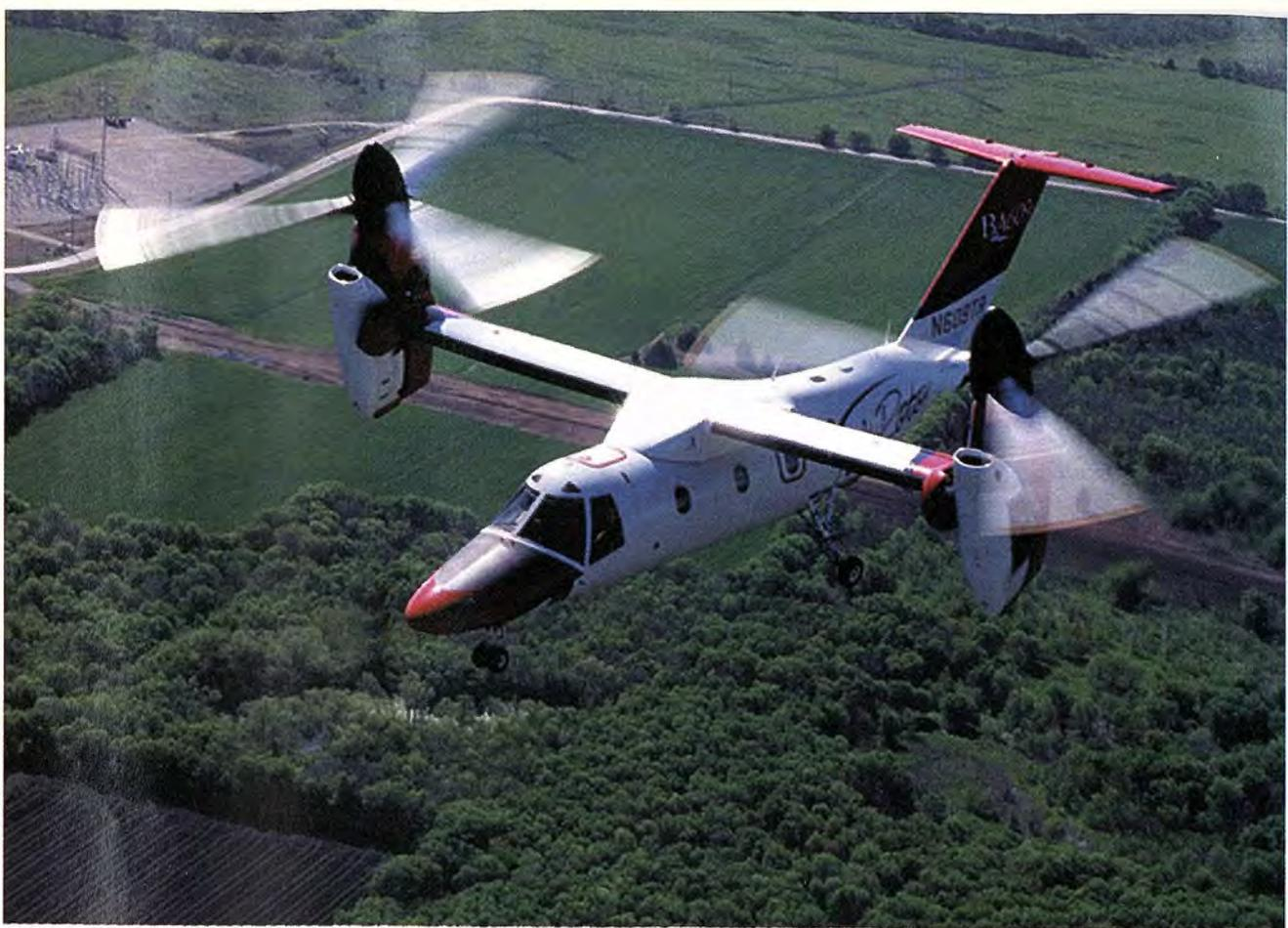
The Bell/Agusta 609 Tiltrotor, from Bell Helicopter, takes off straight up in the air. Rotors then tilt and the craft moves forward. Delivery is set for 2009. To keep this huge project on track, managers follow a blueprint every step of the way, although the plan does include some flexibility.
