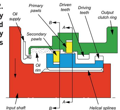
the pawl central pivot pin causes the primary pawls to retract from the ratchet teeth due to centrifugal force when the output exceeds a predetermined speed; typically about 500 rpm.
