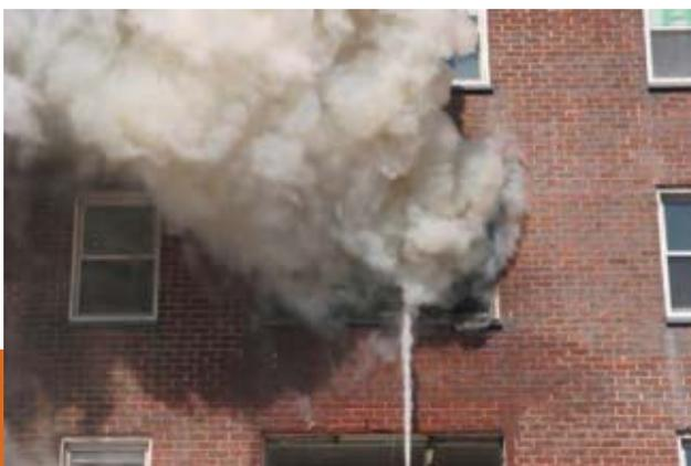
▲ The high-rise nozzle, designed to get water directly onto a fire from the windward side of a building, reduced temperatures in an exposed corridor by 40 percent in about a minute.
