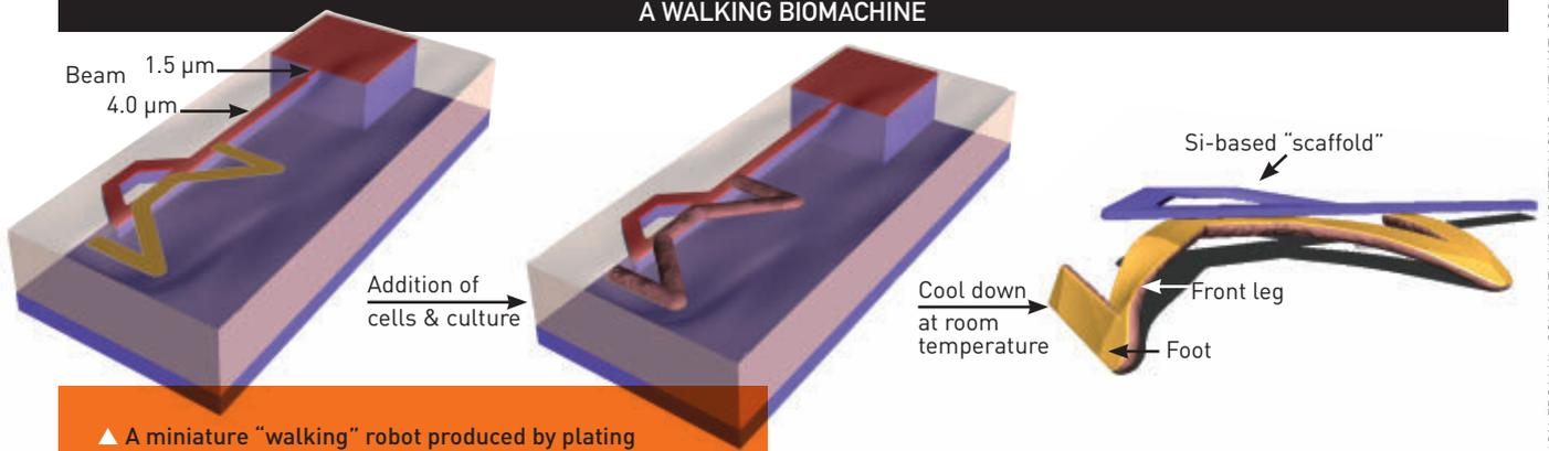
▲ A miniature “walking” robot produced by plating rat neonatal cardiomyocytes onto a flexible substrate, designed so that it crawls along a surface when the muscle periodically contracts and relaxes.
