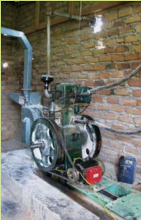
➤ A Listeroid diesel engine that runs on local vegetable oils to mill grain and generate electricity.
