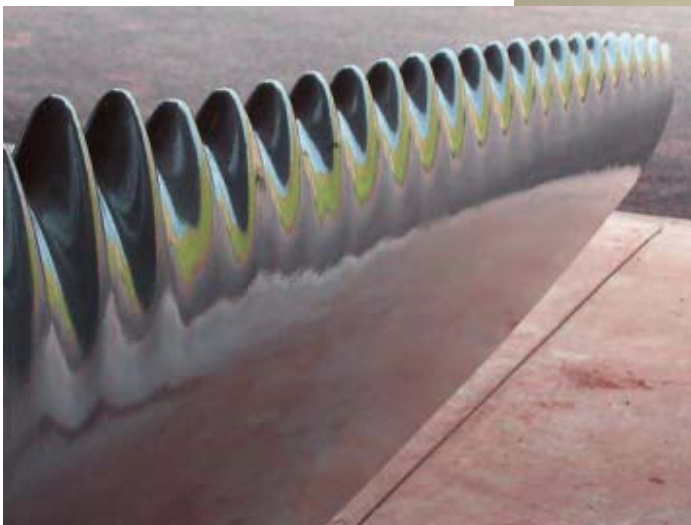
▲ Above, a model of a wind turbine blade with bumps on the leading edge.
