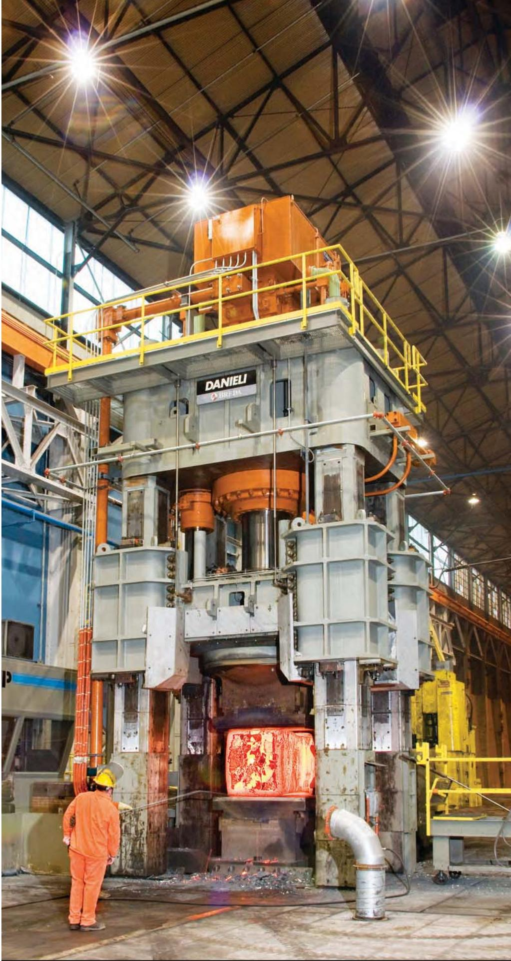
Red-hot ingots (above and left) are being turned into high-quality steel in the 5,000-ton press at Ellwood City Forge's 100,000-square-foot facility in New Castle, Pa.
