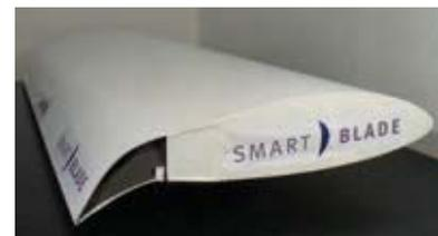
Fig. 1: Wind tunnel test blade with a pneumatically actuated high deflection flexible flap.
