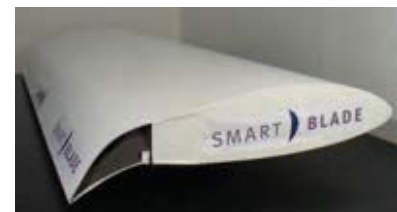
Fig. 1: Wind tunnel test blade with a pneumatically actuated high deflection flexible flap.
