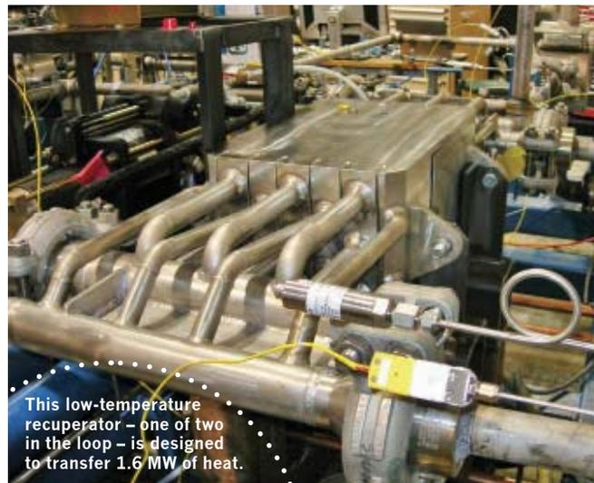
This low-temperature recuperator – one of two in the loop – is designed to transfer 1.6 MW of heat.
