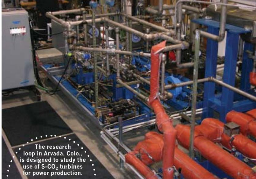
The research loop in Arvada, Colo., is designed to study the use of S-CO<sub>2</sub> turbines for power production.
