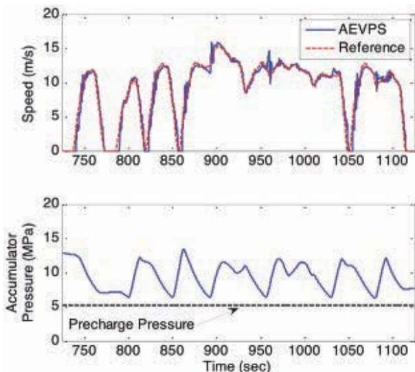
**FIGURE 3** Experimental powertrain response for AEVPS with MPC in urban driving.
