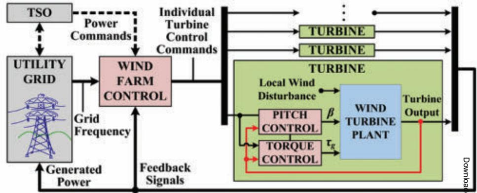
**FIGURE 6** The interconnection between the utility grid, grid operator, wind farm control system, and the individual turbine control system. The wind farm controller measures the grid frequency so that it can provide a primary frequency response (PFR) and receives power commands from the grid operator, for example de-rating commands, power generation schedules, or balancing commands.
