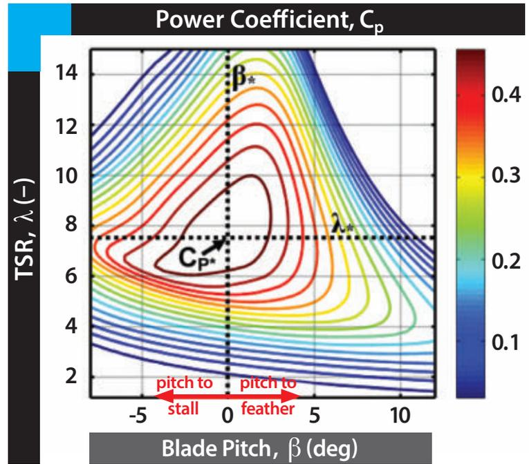
**FIGURE 3** A characterization of the power coefficient  $C_p$  of an example 5MW turbine model. The black dotted lines represent the tip-speed ratio  $\lambda_*$  and the collective blade pitch  $\beta_*$  at which  $C_p$  is a maximum, or  $C_{p*}$ . This plot refers to positive pitch angles as pitching to feather and negative pitch angles as pitching to stall.
