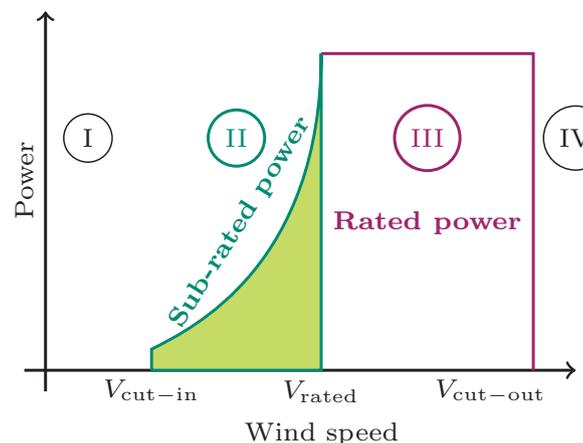
FIGURE 3 Typical power curve of WT including four operating regions.
