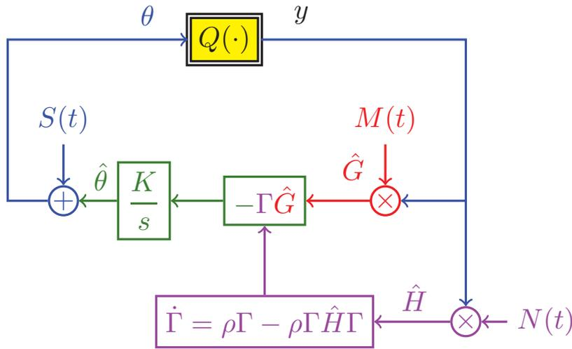
FIGURE 2 A Newton-based ES for a static map.
