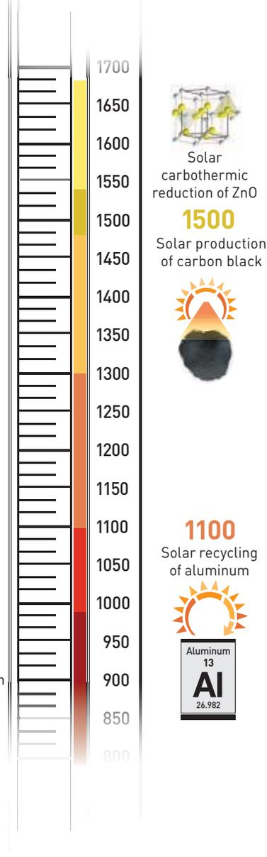
Various thermochemical processes can be driven by the heat obtained via concentrated solar power. Because some reactions are possible through different chemical pathways, there may be more than one temperature at which a commodity material can be produced. (All temperatures in Kelvin.)
