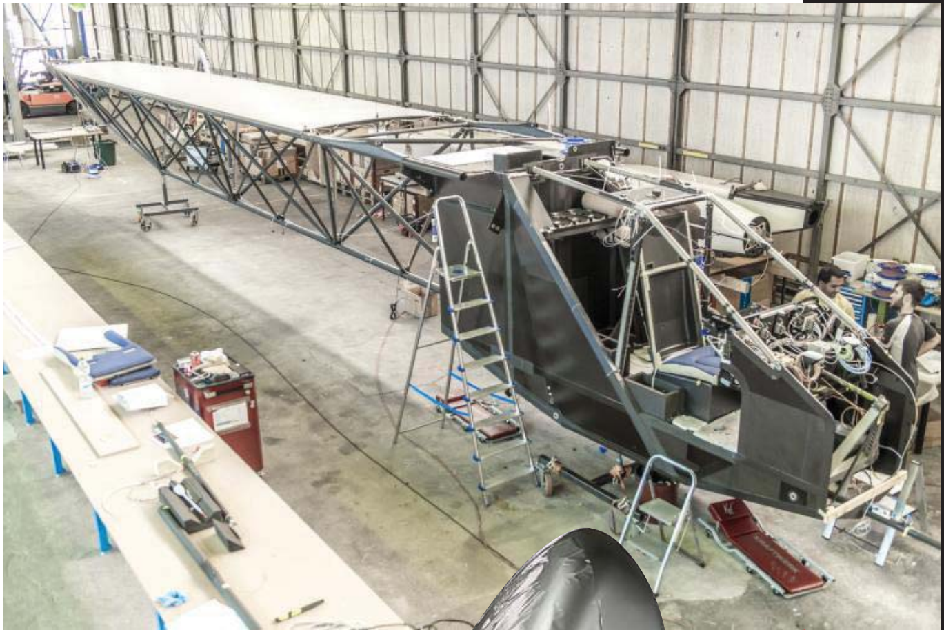
Solar Impulse 2 under construction in Switzerland.
