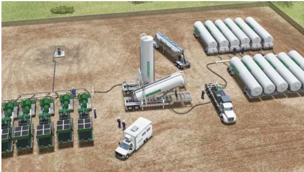
A waterless fracturing operation in progress. Such methods may reduce the perceived environmental impact of "fracking."
