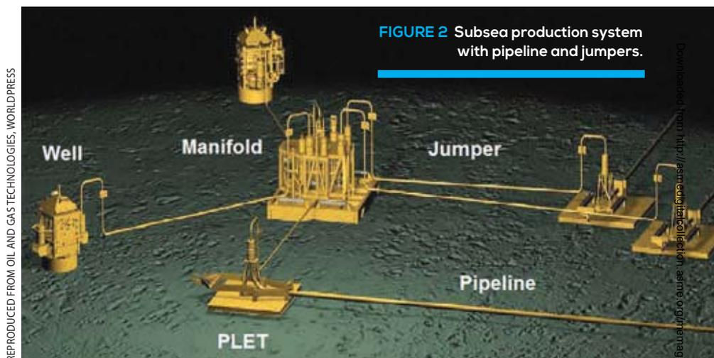
FIGURE 2 Subsea production system with pipeline and jumpers.
