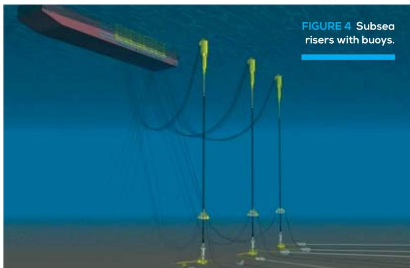
**FIGURE 4** Subsea risers with buoys.
