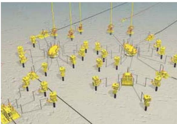
**FIGURE 1** Subsea multi-well and multi-manifold oil and gas production system.
