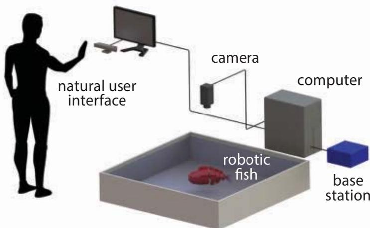
**FIGURE 7** Natural user interface for controlling a robotic fish.
