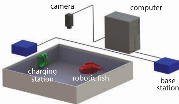
**FIGURE 8** Autonomous charging station for a robotic fish.
