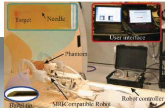
**FIGURE 2** Samples of various MRI-compatible robotic approaches: Clockwise from left: A dexterous neurosurgical robot [Sutherland 2008], A percutaneous needle insertion robot [Stoianovici 2007], and an autonomous image-guided needle steering system [Patel 2015].
