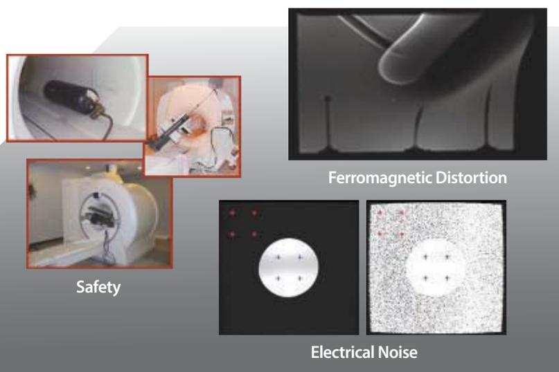
**FIGURE 1** Examples of some of the difficulties encountered with robotics introduced into the MRI environment including safety issue due to projectiles, distortion of the magnetic fields, and introducing electrical noise that degrades image quality.
