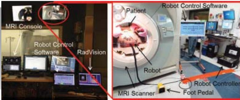
**FIGURE 3** An example of a clinical configuration for MR image-guided prostate cancer biopsy using the robot described in [Eslami 2015].
