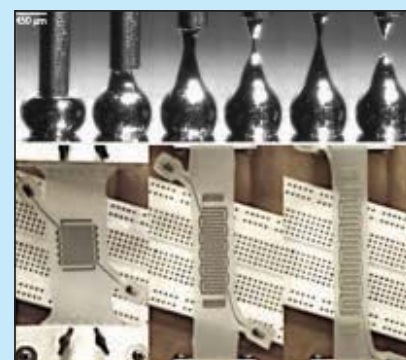
FIGURE 5 (top) Eutectic gallium-indium (EGaIn) alloy is a “moldable” liquid that forms a nanometer-thin oxide skin in air [15]. (bottom) A fluidic channel of EGaIn embedded in silicone deforms with the surrounding elastomer [17].
