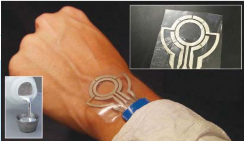
FIGURE 2 Tactile sensor with laser-patterned traces of eutectic gallium-indium (EGaIn) liquid metal (LM) embedded in silicone elastomer.
