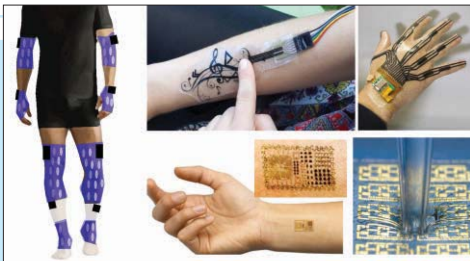
FIGURE 4 Materials and architectures for wearable computing (clockwise from top left): iSkin with conductive silicone elastomer [10]; wireless dataglove with adhesive electronic skin; wavy copper traces for stretchable functionality [11]; UIUC Electronic Tattoo [12].
