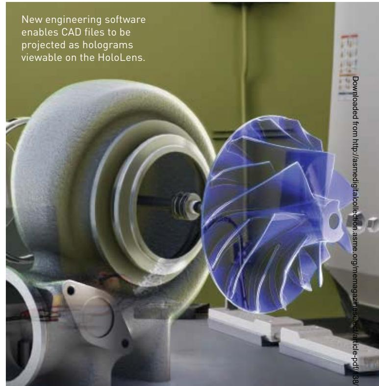
New engineering software enables CAD files to be projected as holograms viewable on the HoloLens.
