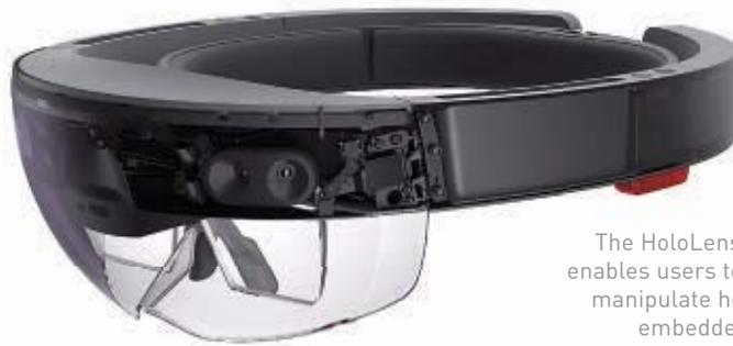
The HoloLens headset enables users to see and manipulate holograms embedded in their environment.
