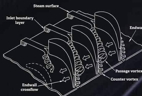
Figure 1. Sketch of a turbine blade cascade with an enhanced rendering of endwall secondary flow [2].
