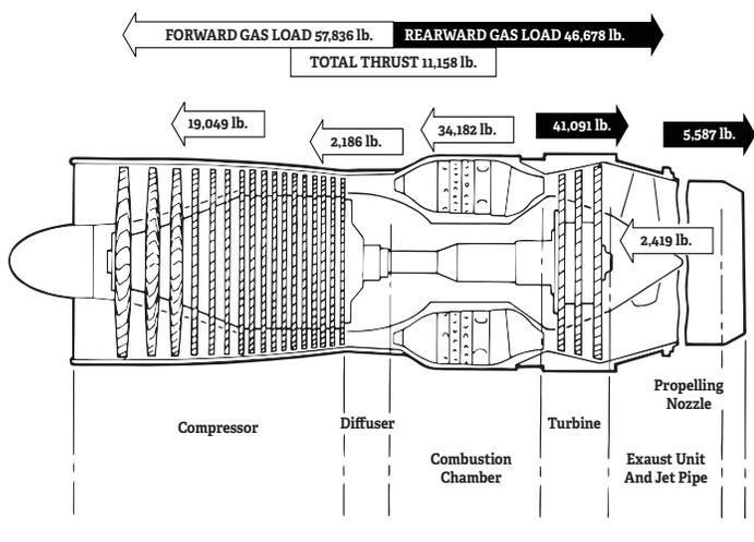
Figure 2. Thrust distribution for a single spool turbojet engine [4].
