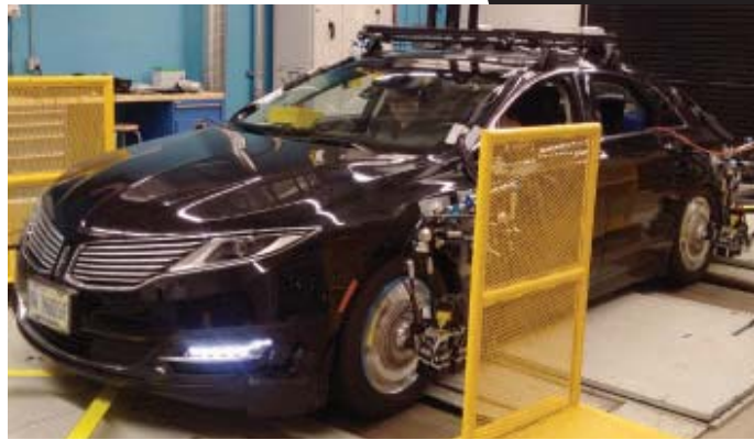
Autonomoose in the GAIA Vehicle Test Cell strapped down and ready to drive-by-wire on the 4-wheel chassis dynamometer. Autonomoose, a Lincoln MKZ hybrid, is Canada's first autonomous vehicle.
