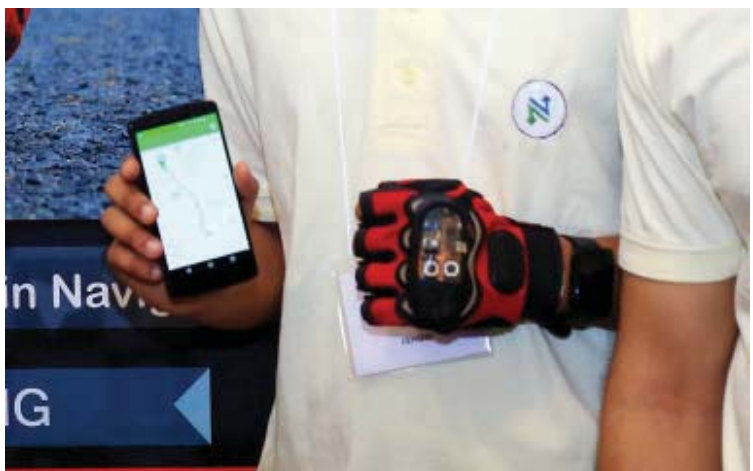
Engineers compete in ASME’s IShow India. The international hardware competition features many solutions that include IoT-related technologies. Above is Navyo, a Bluetooth-connected smart glove accompanied by a Mobile App that can guide a blind person turn by turn via vibrations.
