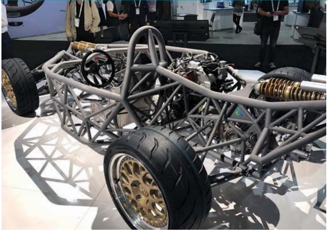
The chassis of La Bandita Speedster was generatively designed to support a shape sculpted in virtual reality.
