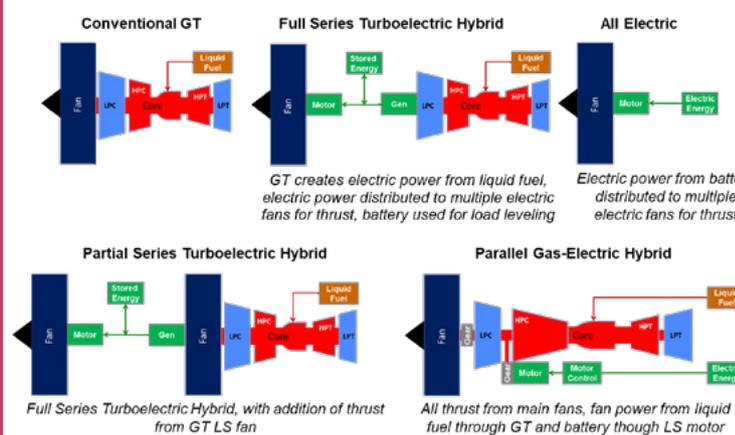
Figure 1. Electrified Propulsion Architectures
