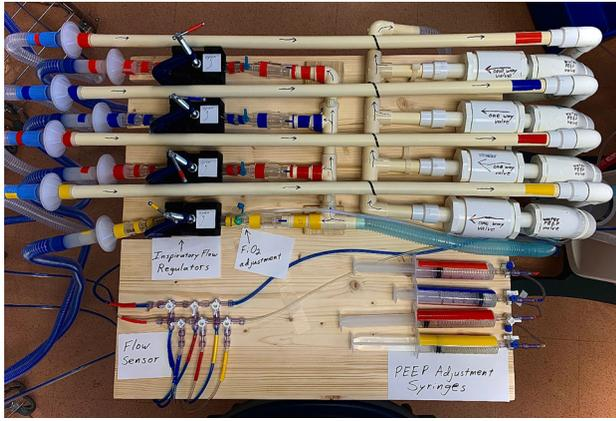
**Fig. 2 MSVS system assembled using commonly available components**
