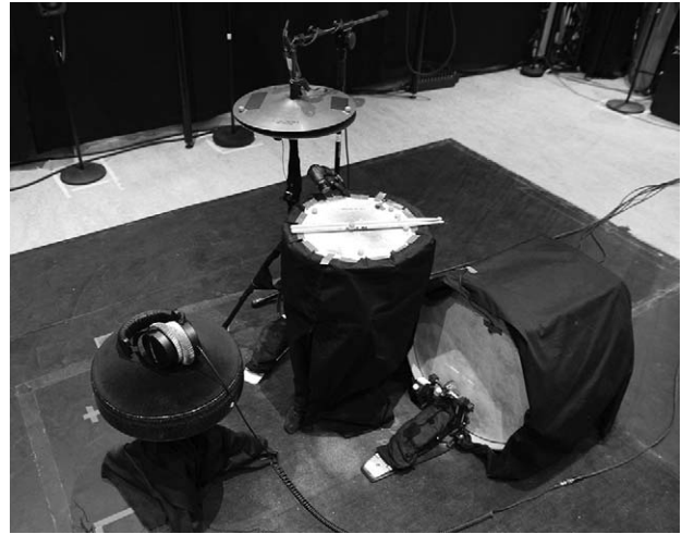
FIGURE 2. Drum-kit setup. Drum-kit covered in black textile in order to avoid problems with reflections in the motion-capture recordings.
