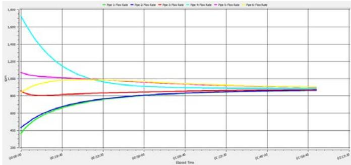
FIGURE 3. TANK FLOW RATES WITH ALL TANKS CROSS CONNECTED
