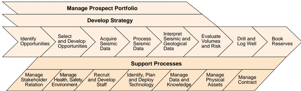
**Figure 4: This exploration work-flow allows for early generation and selection of new play concepts and opportunities, utilizing existing and newly acquired seismic, well and geological data.**
