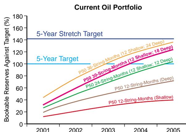
**Figure 8:** Simulation results used to assess the optimum drilling intensity and rig composition.
