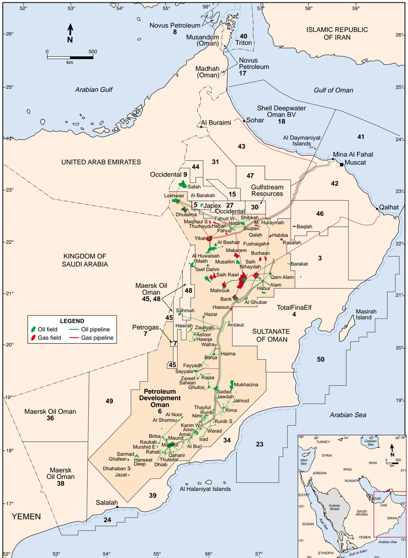
Figure 1: PDO concession map indicating location of producing fields and pipeline infrastructure.
