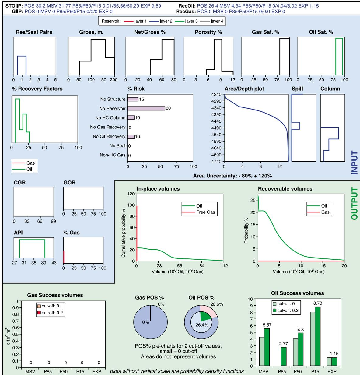
**Figure 6: Screen display example of Excel summary sheet displaying prospect characteristics input and volumetric output. This kind of summary enables a quick quantitative assessment of the volumetrics and risk of an exploration opportunity. Input is shown in blue and output in green.**
