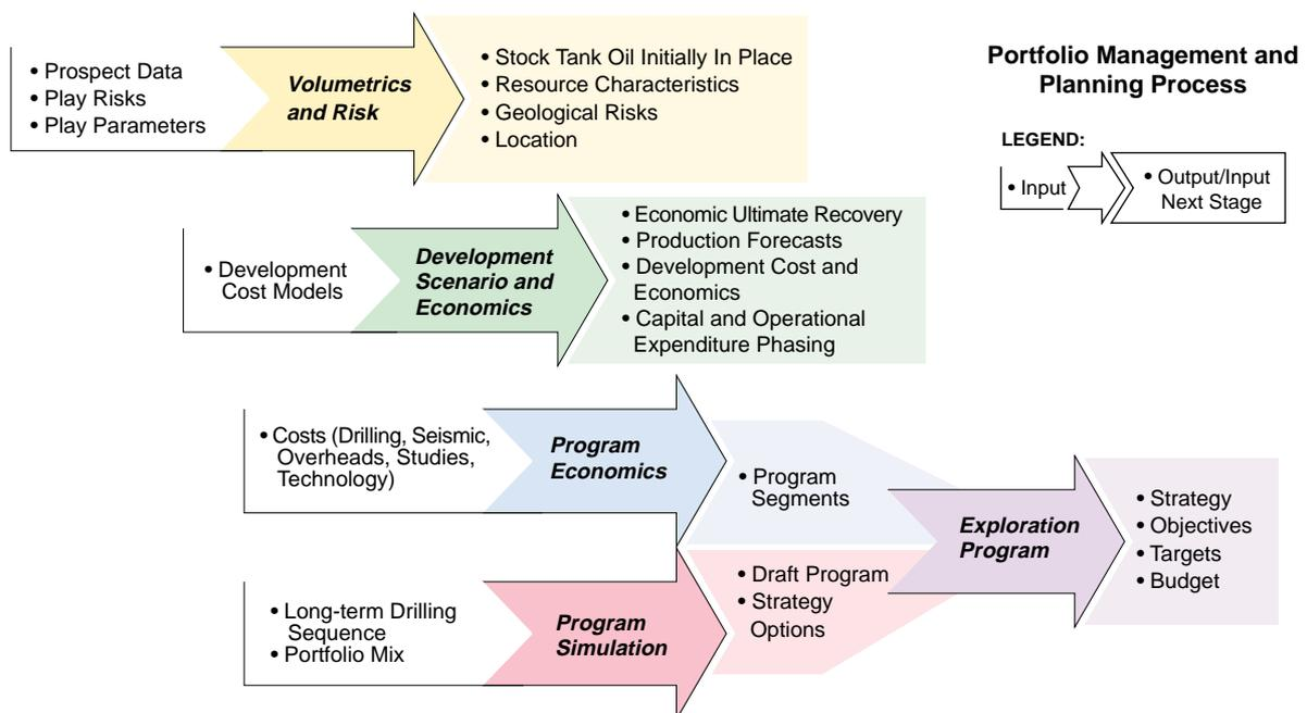
**Figure 5: The sequence of tools used in the process flow from volume to value assessments. Tools are shown as colored arrows, adjacent to the key input and output parameters.**
