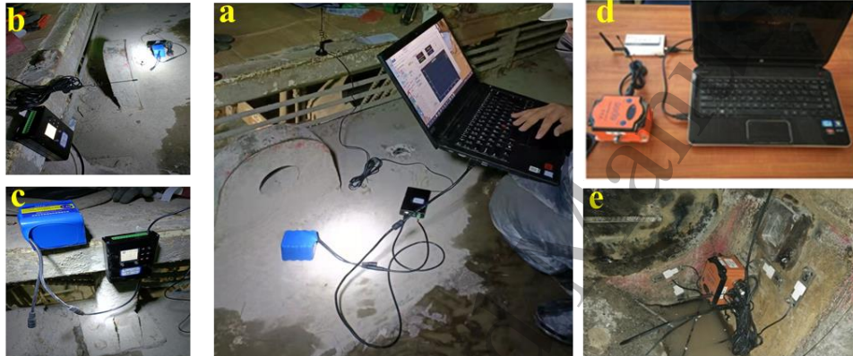
Figure 6 Field verification of engineering example. (a) On-site commissioning and installation stage, (b) Acquisition and monitoring wireless module, (c) In-situ monitoring system, (d) Remote online monitoring by the host computer, (e) The key structural position of the installation equipment of the strain monitoring package node.
