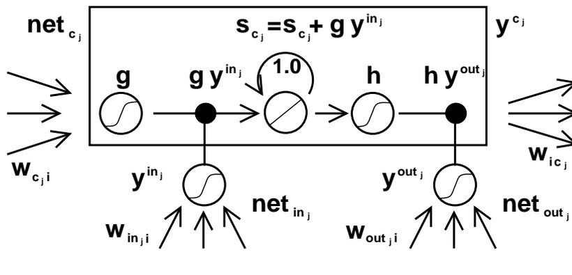
Figure 1: Architecture of memory cell  $c_j$  (the box) and its gate units  $in_j$ ,  $out_j$ . The self-recurrent connection (with weight 1.0) indicates feedback with a delay of one time step. It builds the basis of the CEC. The gate units open and close access to CEC. See text and appendix A.1 for details.
