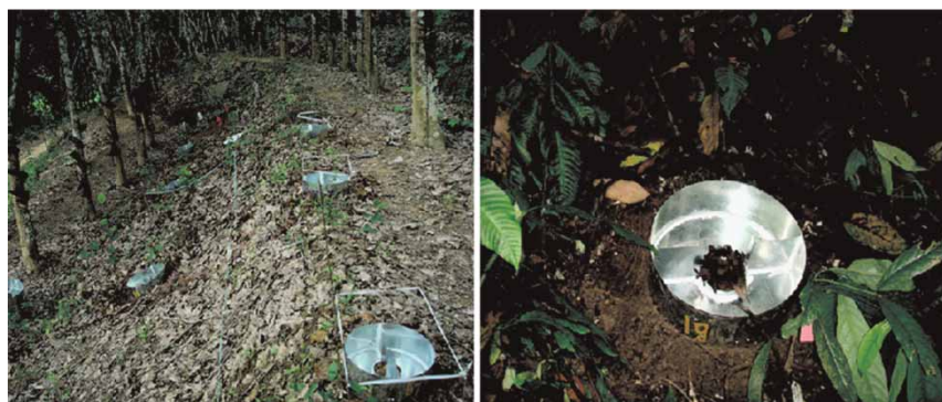
Figure 1 | Morgan-type splash cups installed on the floor to collect soil sediment splashed from the ground surface in the bench-terraced rubber plantation (left) and the tropical rainforest (right).
