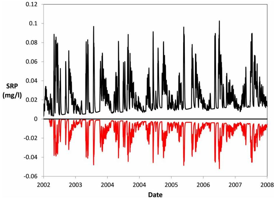
**Figure 6** | INCA-P output for River Tywi showing baseline superphosphate (black line) and expected reduction in SRP that could be achieved with 50% of inorganic P fertilizer replaced with biosolids (digested cake).
