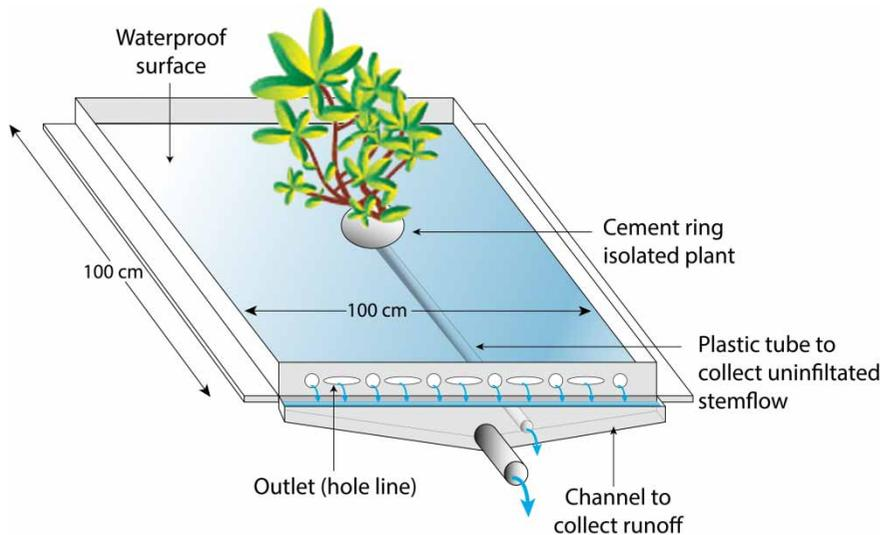
**Figure 2** | Metal frame and runoff tube collectors for each 1 m<sup>2</sup> plot used for the rainfall simulations.
