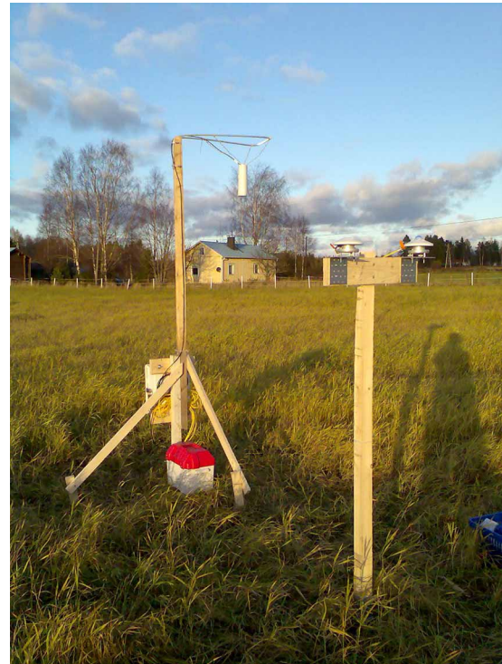
Figure 1 | Setup of the radiation and temperature observational station at the open field site in Evo, southern boreal Finland.
