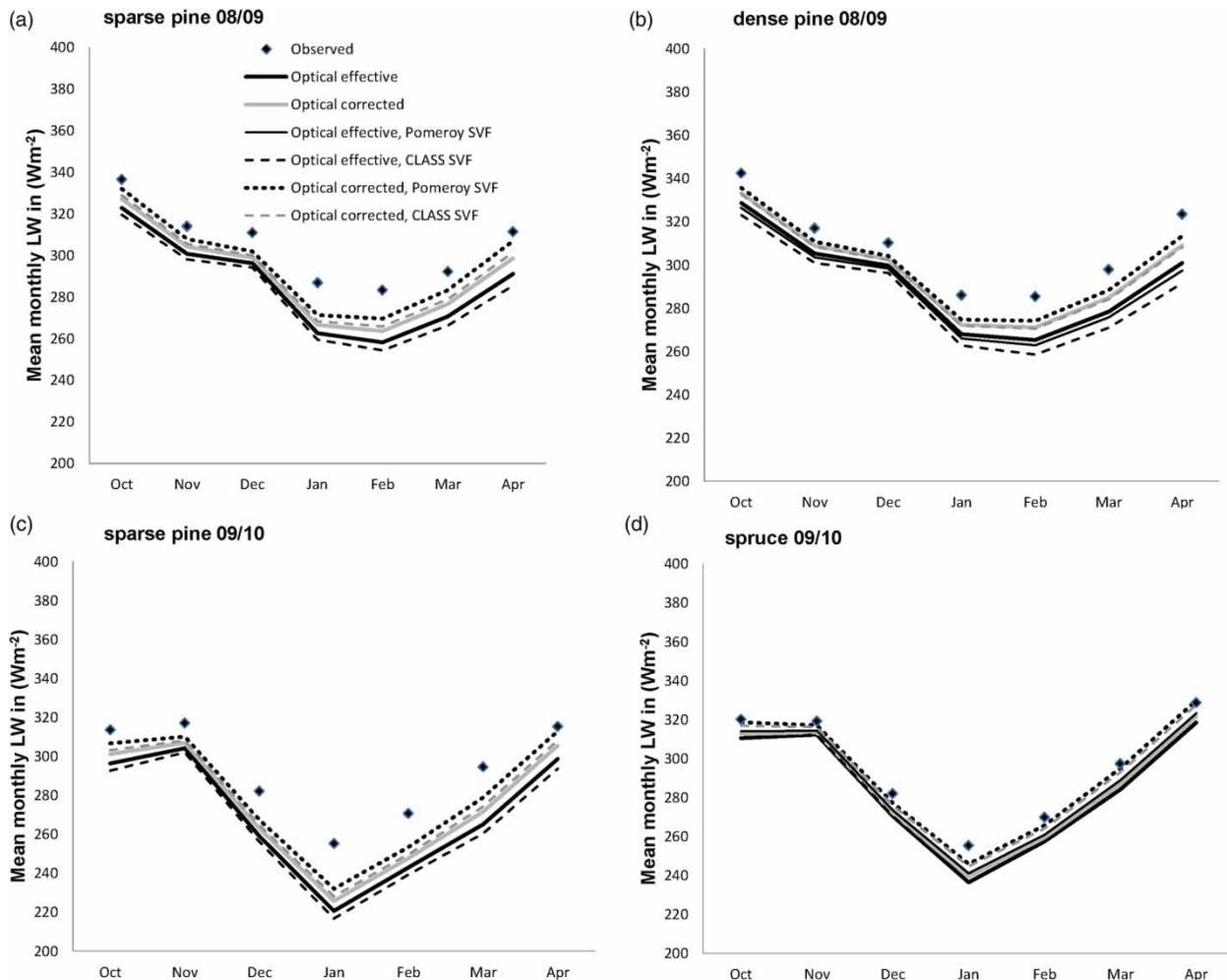
**Figure 8** | Simulated mean monthly incoming longwave radiation using the LAI and canopy openness (SVF) parameterizations listed in Table 1 during winter 2008–2009 in the pine forest with (a) sparse canopy and (b) dense canopy, and during winter 2009–2010 in the (c) sparse pine forest and in the (d) spruce forest. Dots mark the observations from the site.
