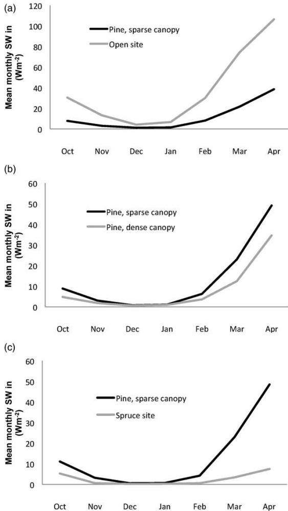
**Figure 3** | Observed mean monthly incoming shortwave radiation in the open field and (a) below the sparse pine canopy during the winter 2007–2008, (b) below the sparse and the dense pine canopy during the winter 2008–2009 and (c) below the sparse pine and the spruce canopy during the winter 2009–2010.
