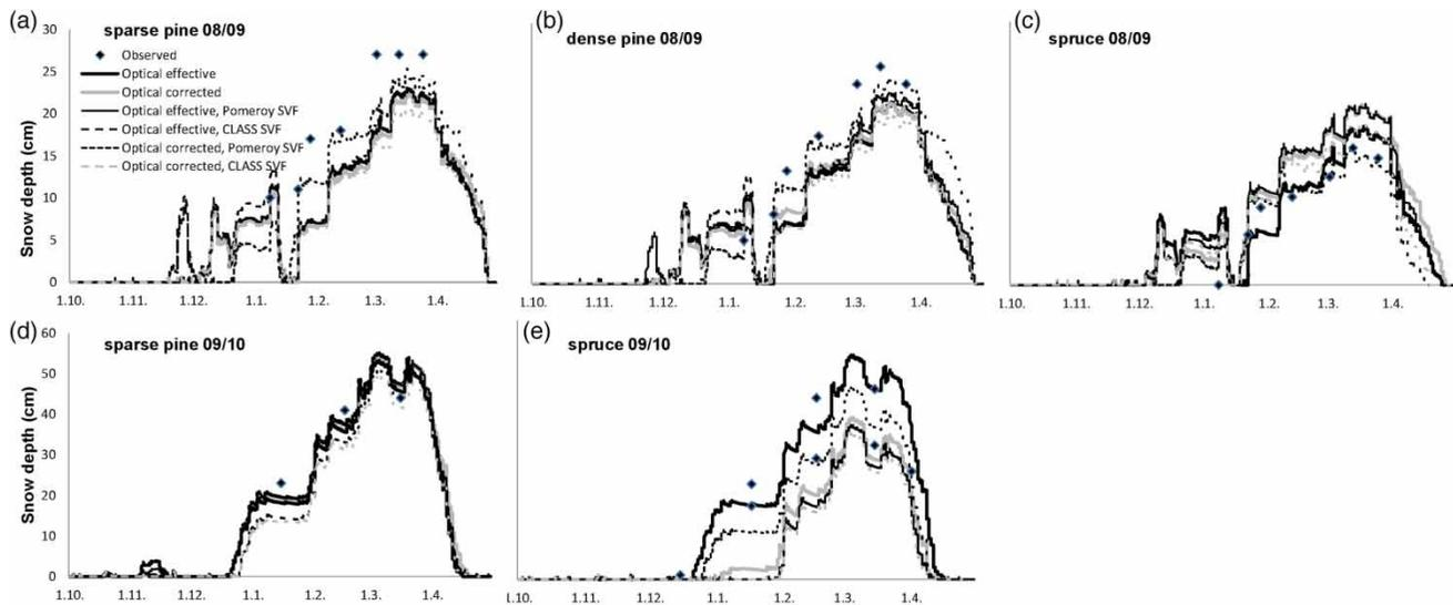
**Figure 5** | Simulated snow depths using the LAI and canopy openness (SVF) parameterizations listed in Table 1: winter 2008–2009, (a) sparse pine; (b) dense pine and (c) spruce canopy; winter 2009–2010, (d) sparse pine and (e) spruce canopy. Dots mark the observations from the site.
