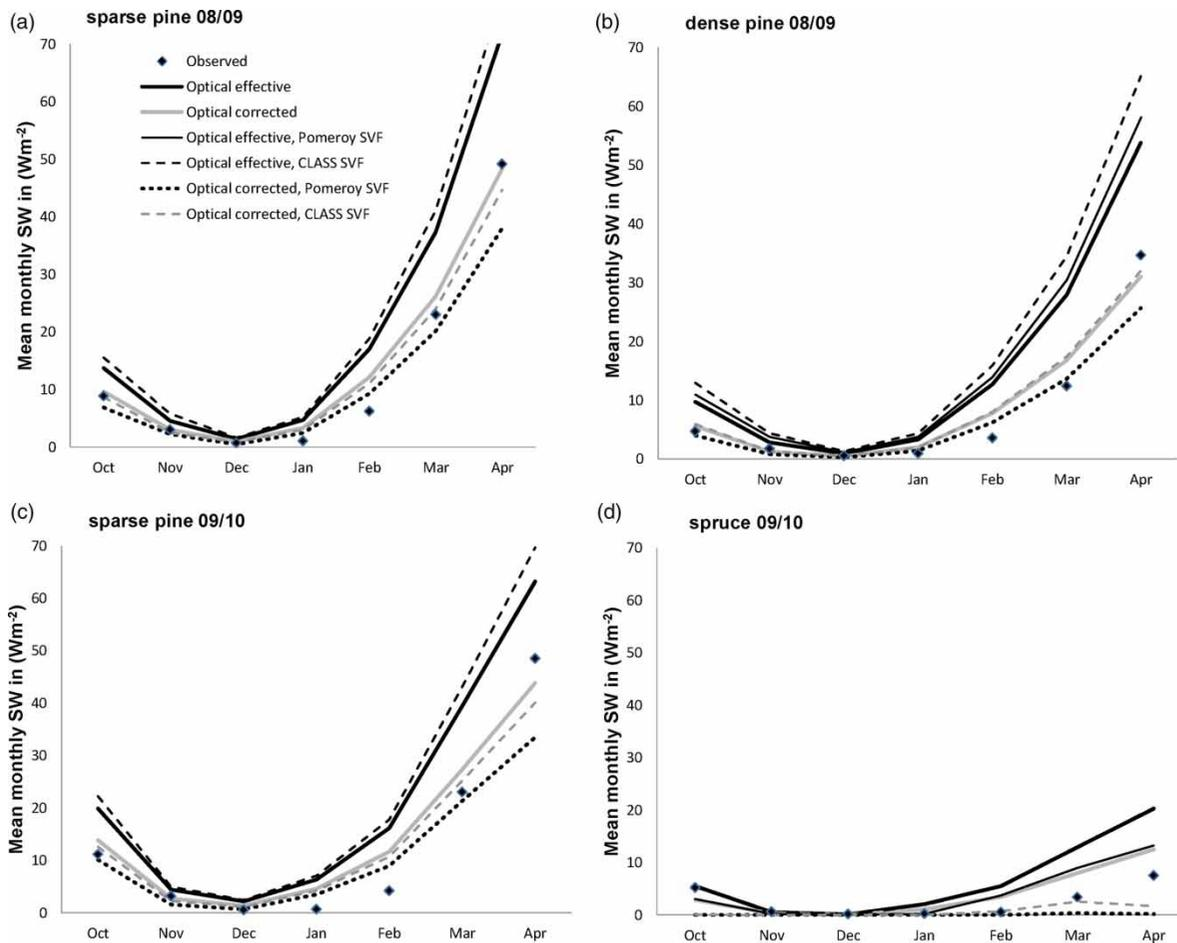
**Figure 7** | Simulated mean monthly incoming shortwave radiation using the LAI and canopy openness (SVF) parameterizations listed in Table 1 during winter 2008–2009 in the pine forest with (a) sparse canopy and (b) dense canopy and during winter 2009–2010 in the (c) sparse pine forest and in the (d) spruce forest. Dots mark the observations from the site.
