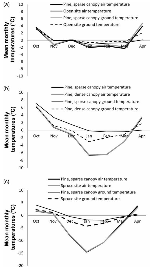
**Figure 2** | Observed mean monthly air and snow–soil interface temperatures in the open field and (a) below the sparse pine canopy during the winter 2007–2008, (b) below the sparse and the dense pine canopy during the winter 2008–2009 and (c) below the sparse pine and the spruce canopy during the winter 2009–2010.
