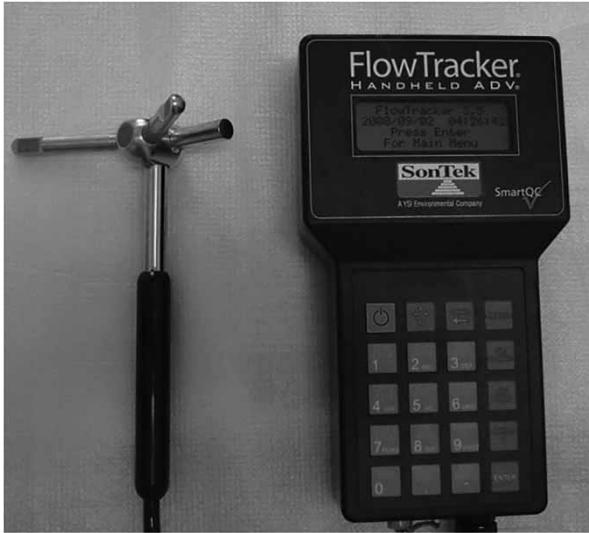
Figure 3 | Acoustic Doppler velocimeter, Sontek FlowTracker.
