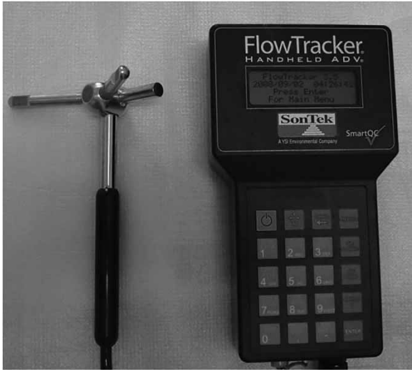
Figure 3 | Acoustic Doppler velocimeter, Sontek FlowTracker.
