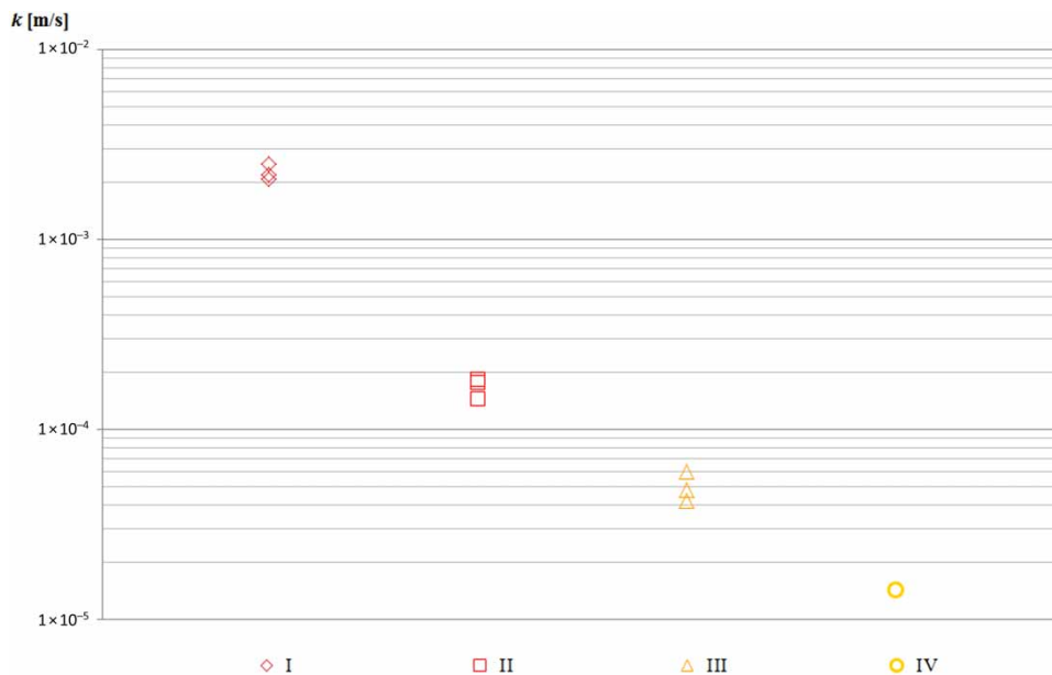
Figure 3 | Hydraulic conductivity measurements performed in the W-tube for all tested sand samples.
