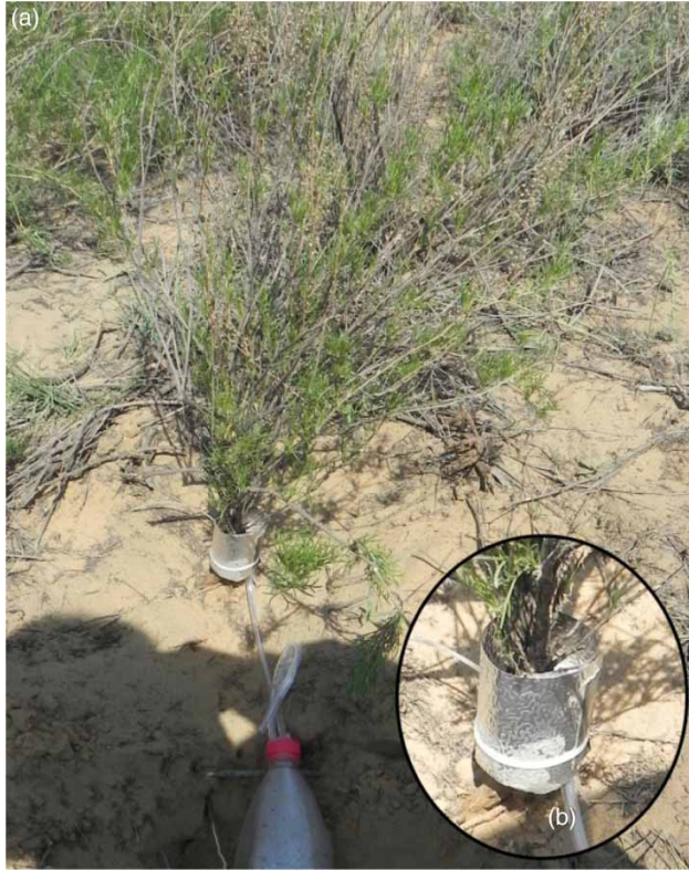
Figure 1 | (a) Artemisia ordosica subshrub; and (b) stemflow collection apparatus on trunk of an experimental individual.
